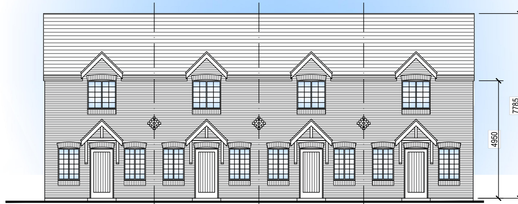
Elevation 2 - front elevation 1:100 0 5 scale Facing brick to be orange/red to match existing main house. Tiles to be grey tiles to match existing main house. Brick soldiers to window heads and cills.
